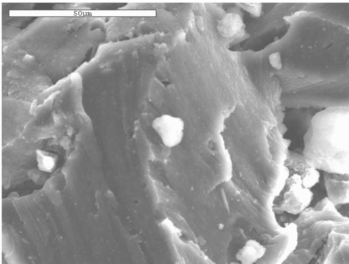
**Figure 2** SEM micrograph of rubber dust samples removed from the factory. Note: the small white particle in the center of the photograph is a piece of the silica powder used as an anti-clumping agent.
