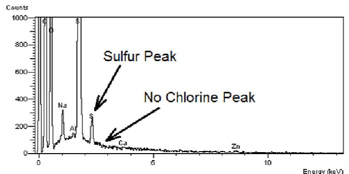
**Figure 3.** EDS Spectrum obtained from silica particles in a randomly selected rubber dust sample removed from the exploded factory. The absence of a chlorine peak indicates a different product supplier than the one named in the lawsuit.
